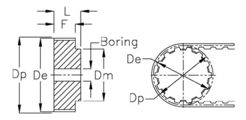
Belt width Type = T5= - 16 mm Weight = 0.43= 75.55 De Dm = 50 = 76.55 Dp F = 21 L = 27 Pre-drilled = 8 Tooth number = 48
